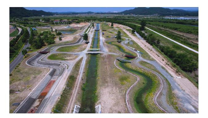
The River Experiment Center in Andong has three straight and curved experimental water channels with dimensions of 700m(L)\*11m(W)\*2m(H), and operates a laboratory for empirical testing of dike failure and urban flood defense technologies. Credit: Korea Institute of Civil Engineering and Building Technology
