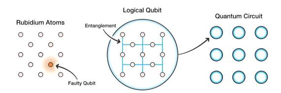
Individual physical qubits, like rubidium atoms, are notoriously fragile and easily disturbed by interactions with their environment. To minimize errors, researchers entangle the atoms together to form a single "logical qubit," which can be combined with other logical qubits into a fault-tolerant quantum circuit. Credit: S. Kelley/NIST
