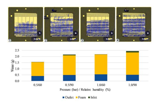
Effect of relative humidity and pressure on water distribution (T=65°C, CD=1 A/cm<sup>2</sup>). Liquid water distribution in the cell from neutron radiographies of the experiments 1, 2, 3 and 4 (top), and amount of water in the cell (bottom). Credit: *International Journal of Hydrogen Energy* (2023). DOI: 10.1016/j.ijhydene.2023.08.103
