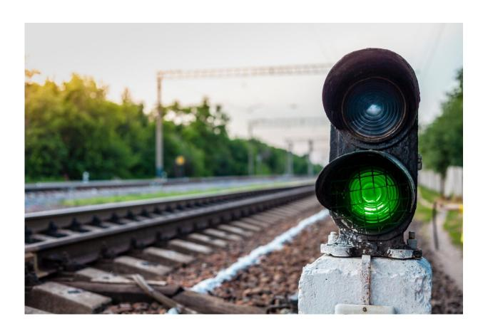
"Wrong side" failures—when the signal goes from red to green—are much more hazardous than "right side" failures which are green to red. Credit: Lancaster University
