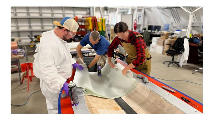
After optimizing it in the lab, the NREL team used their new PECAN resin to glue together a 9-meter wind turbine blade made with fiberglass composites and a balsawood core in NREL's Composites Manufacturing Education and Technology Facility. Credit: Troy Boro, NREL
