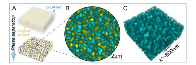
A piece of polymer is placed in an oily solution and heated. This causes the polymer and the oil to blend and form a network. If the material is subsequently cooled down to room temperature, it is possible to identify the network created by the phase separation. Credit: *Nature Materials* (2023). DOI: 10.1038/s41563-023-01703-0
