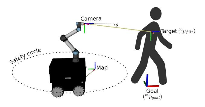
Overview of relevant transformation frames and representation of the safety circle used during the FollowMe application. Credit: Rollo et al.
