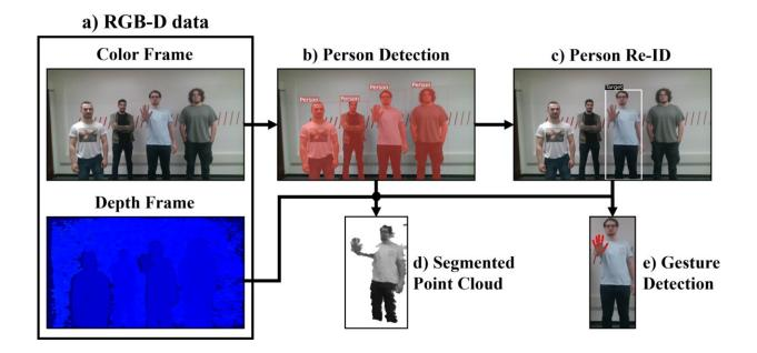
Perception pipeline: (a) RGB and Depth image acquisition; (b) person detection through Yolact++ (see Sect. III-A); (c) person Re-ID using deep neural network and human features distance ; (d) person localization using the point cloud and Re- Identified person mask; (e) gesture detection to send commands to the robot. Credit: Rollo et al.
