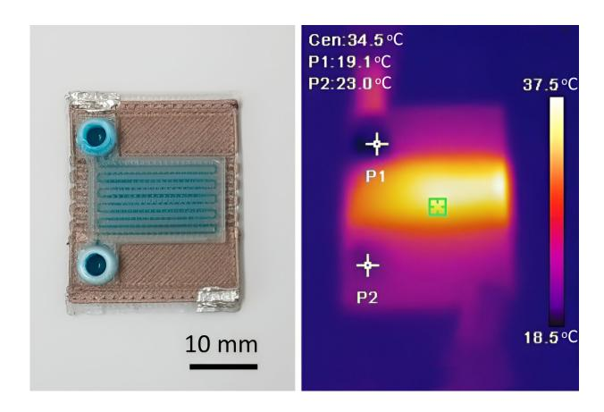
MIT researchers developed a fabrication process to produce self-heating microfluidic devices in one step using a multi-material 3D printer. Pictured is an example of one of the devices. Credit: Massachusetts Institute of Technology
