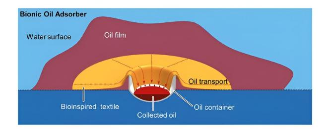
Cross-section of computer-aided (CAD) model of the Bionic Oil Adsorber Credit: ITA
