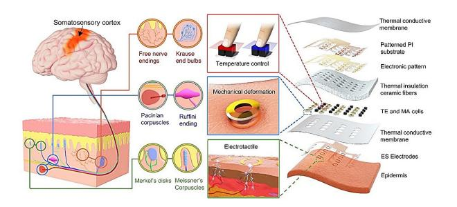
Schematic of the neural tactile sensing system and corresponding three stimulation modes. An exploded-view illustration of a device with 16 independently controlled multimodal haptic feedback units, each unit has a mechanical actuator (MA), two pairs of thermoelectric (TE) pellets and one pair of electrotactile (ES) electrodes. Credit: Huang et al.
