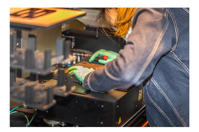
A UNSW researcher measuring the current-voltage characteristics of an industrial TOPCon silicon solar cell. Credit: Bram Hoex/University of New South Wales
