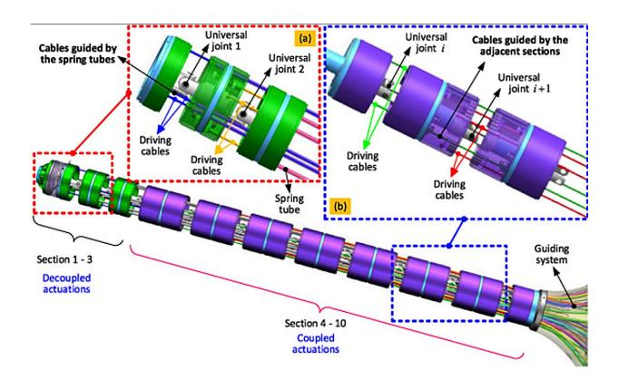
Schematic of the 20 DoF snake robot showing the structure for the "macro–micro" operation: (a) shows the three tip sections with decoupled actuation; (b) shows the seven base sections with coupled actuation. Credit: Ma et al
