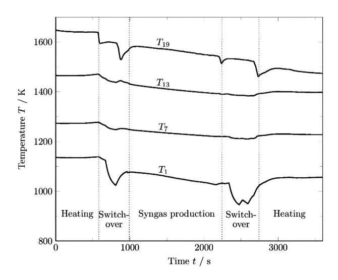
Temperature development over time in cyclic operation for 4 chosen temperature sensors along the reforming channel. Credit: *Energy Advances* (2023). DOI: 10.1039/D3YA00227F
