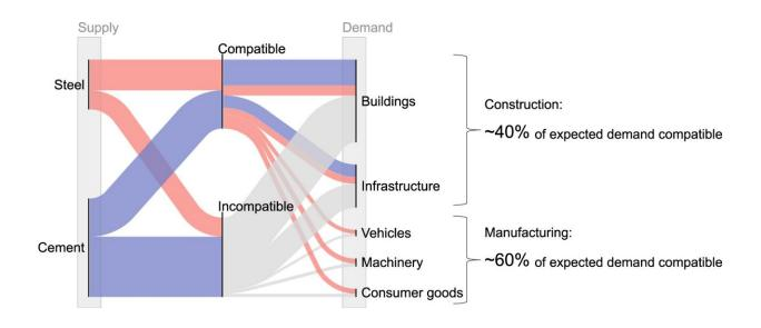
Comparison of the global feasible supply and expected demand for the construction and manufacturing sectors in 2050. Credit: *Nature Communications* (2023). DOI: 10.1038/s41467-023-43684-3
