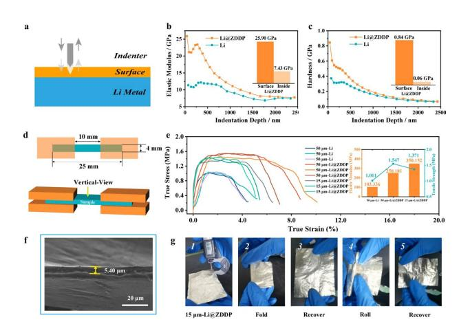
Mechanical properties of Li@ZDDP strips. a Schematic diagram of cyclic loading mode for nanoindentation test. b Comparisons of elastic modulus between bare Li metal and Li@ZDDP films using nanoindentation measurements. c Comparisons of hardness between bare Li metal and Li@ZDDP films using nanoindentation measurements. d Dimensional drawing
