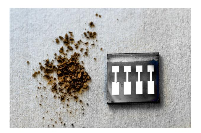
Kraft lignin improves the stability in organic solar cells thanks to its ability to form hydrogen bonds that acts as a sort of glue. Credit: Thor Balkhed
