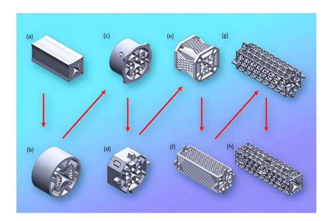
Because additive manufacturing allows the researchers to easily try new designs, they created a number of different quadrupole filters before arriving at the final iteration (h), which is surrounded by a series of triangular lattices to provide durability. Credit: Massachusetts Institute of Technology
