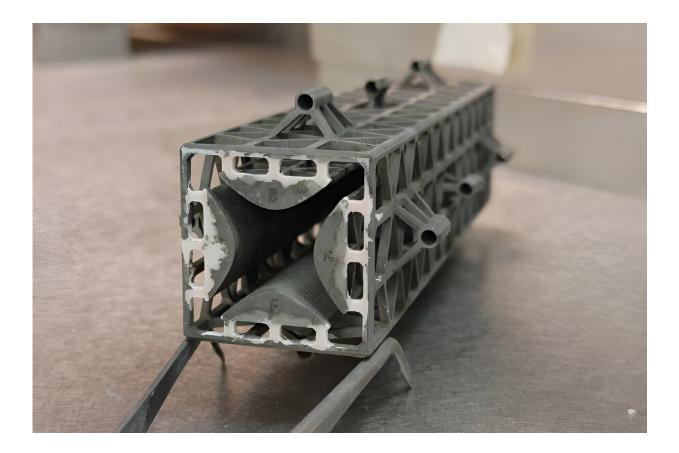
An example of a 3D printed miniaturized quadrupole mass filter. They can be fabricated in a matter of hours for a few dollars. Credit: Colin C. Eckhoff et al
