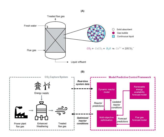
Schematic representation of (A) enhanced weather packed bubble column reactor and (B) the model predictive control framework developed to maximize
