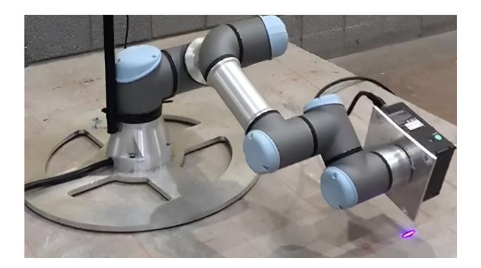
Drexel researchers have created a multi-scale system that uses computer vision and machine learning programs to identify cracks in concrete and direct robotic scanning, modeling and monitoring. Credit: Drexel University
