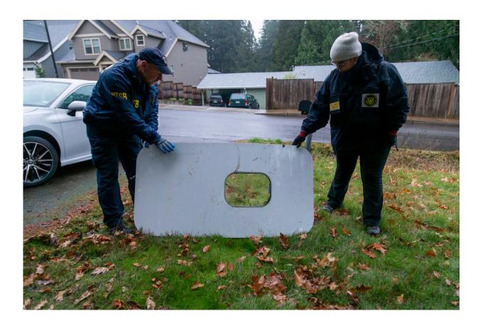
This photo released by the National Transportation Safety Board shows the door plug from Alaska Airlines Flight 1282 on Monday, Jan. 8, 2024, in Portland, Ore. A panel used to plug an area reserved for an exit door on the Boeing 737 Max 9 jetliner blew out Jan. 5, shortly after the flight took off from Portland, forcing the plane to return to Portland International Airport. Credit: National Transportation Safety Board via AP
