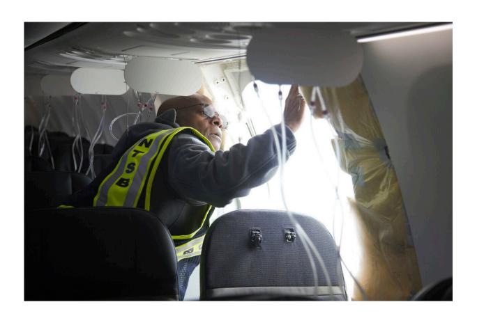
In this photo released by the National Transportation Safety Board, NTSB Investigator-in-Charge John Lovell examines the fuselage plug area of Alaska Airlines Flight 1282 on Sunday, Jan. 7, 2024, in Portland, Ore. A panel used to plug an area reserved for an exit door on the Boeing 737 Max 9 jetliner blew out Friday night shortly after the flight took off from Portland, forcing the plane to return to Portland International Airport. Credit: National Transportation Safety
