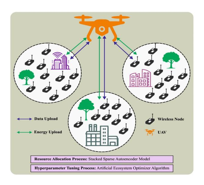
Overall procedure of the IRA-AEODL system. Credit: *Drones* (2023). DOI: 10.3390/drones7100619
