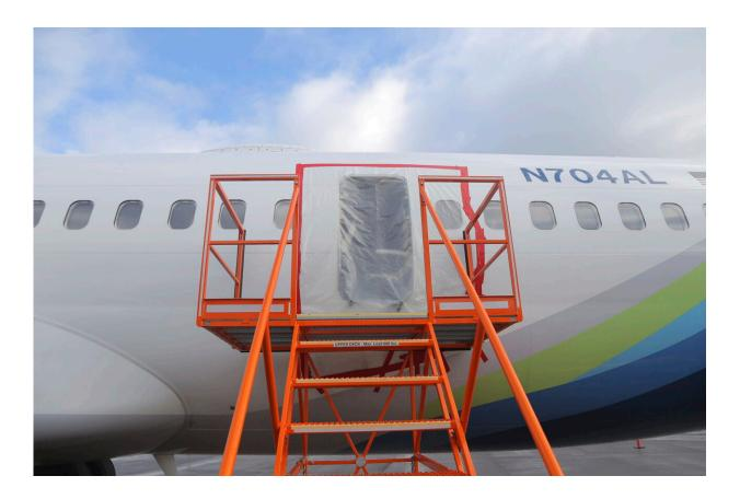
This photo released by the National Transportation Safety Board shows a gaping hole where the paneled-over door had been at the fuselage plug area of Alaska Airlines Flight 1282 on Sunday, Jan. 7, 2024, in Portland, Ore. A panel used to plug an area reserved for an exit door on the Boeing 737 Max 9 jetliner blew out Jan. 5, shortly after the flight took off from Portland, forcing the plane to return to Portland International Airport. Credit: National Transportation Safety Board via AP
