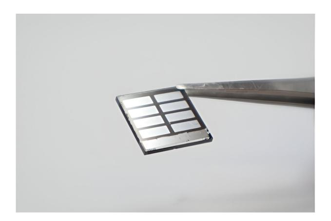
Perovskite solar cells like this one, made by Xiwen Gong's group, could make solar energy cheaper and more environmentally friendly—but they degrade faster than silicon. In a study published in the journal Matter, the team discovered how to make the black perovskite film last longer. Photo credit: Zhengtao Hu, Gong Lab, University of Michigan.
