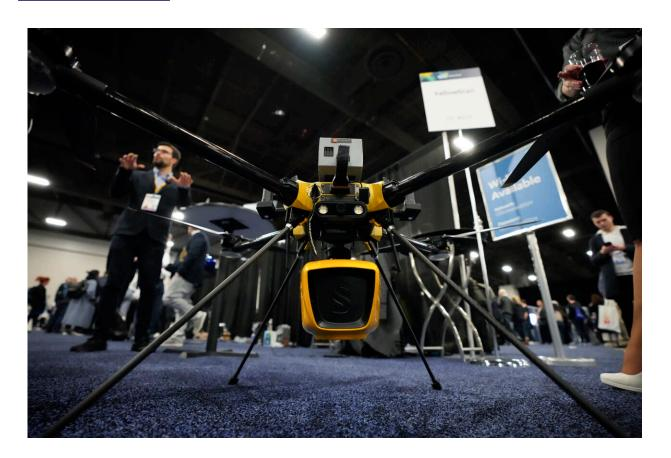
A YellowScan Navigator bathymetric LiDAR system is seen attached to a drone during CES Unveiled before the start of the CES tech show Sunday, Jan. 7, 2024, in Las Vegas. The system is designed for surveying land and waterbeds. Credit: AP Photo/Ryan Sun
