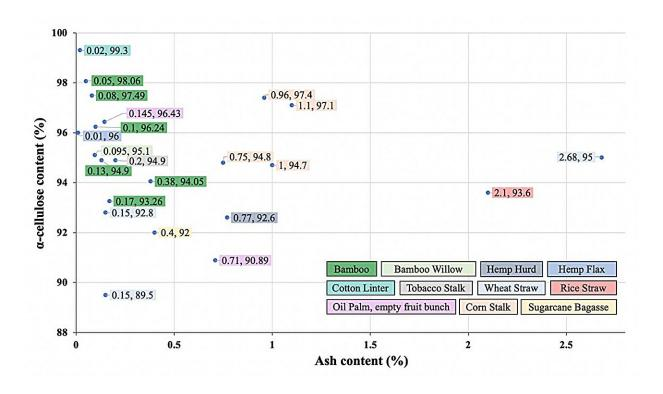
Dissolving pulp  $\alpha$ -cellulose and ash contents achieved by various alternative feedstock and pulping combinations (globally). High  $\alpha$ -cellulose values combined with low ash contents yield pulp most suitable for textile conversion. Note, this graphic does not consider availability. Credit: Ryen Frazier. Credit: Ryen M. Frazier, Department of Forest Biomaterials, North Carolina State University, Raleigh, NC 27695, U.S.
