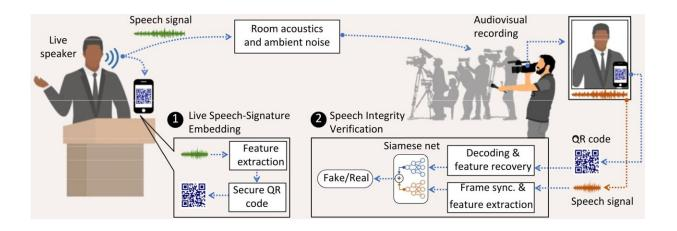
A diagram overview of how TalkLock works. Users can embed a secure QR code in a live recording of an event in real-time and later verify other multimedia content against this code. Credit: Nirupam Roy
