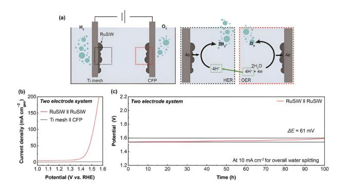
Overall water splitting using RuSiW as a bifunctional HER and OER catalyst. (a) Experimental scheme. (b) Polarization curves of the full cells: RuSiW on CFP as an anode, RuSiW on Ti mesh as a cathode, and 0.5 m  $H_2SO_4$  as an electrolyte. (c) Chronopotentiograms of the corresponding full cells at 10 mA cm<sup>-2</sup>. Credit: UNIST
