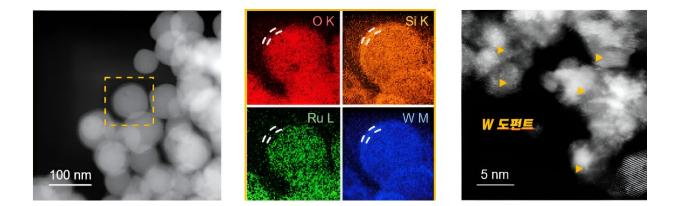
Schematic image showing the characteristics of RuSiW. (Left) Dark-field STEM, (Center) EDX elemental mapping images of RuSiW, and (Right) High-resolution bright-field TEM image of RuSiW. Credit: UNIST
