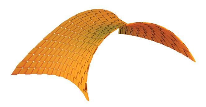
A newly patented kind of energy generator could be woven into fabrics, building walls, or roads to form what their inventors call "metamaterials." As wind, waves, or the pressure of a car deforms these electric quilts, individual generators create sparks of energy. Credit: Besiki Kazaishvili, NREL
