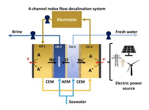
Schematic for a four-channel RFD in single-pass mode with an A/A\*, representing electrochemical reactions of redox species dissolved in conducting salts solutions, and channels separated by cation-exchange membrane (CEM) and anion-exchange membrane (AEM). Credit: NYU Tandon School of Engineering
