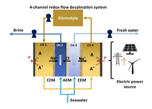
Schematic for a four-channel RFD in single-pass mode with an A/A\*, representing electrochemical reactions of redox species dissolved in conducting salts solutions, and channels separated by cation-exchange membrane (CEM) and anion-exchange membrane (AEM). Credit: NYU Tandon School of Engineering
