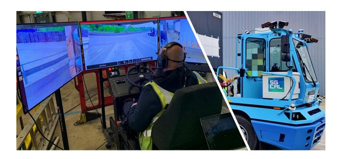
An example of a remote driver operating a teleoperation workstation for remote driving (left) of a 5G-enabled Level 4 automated vehicle (right) in the DCMS 5G Connected Automated Logistics project. Credit: *Transportation Research Part F: Traffic Psychology and Behaviour* (2023). DOI: 10.1016/j.trf.2023.11.018
