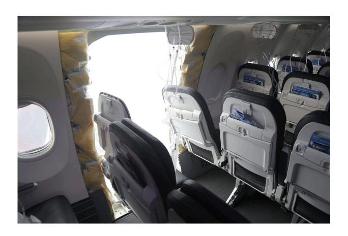
This image taken Sunday, Jan. 7, 2024, and released by the National Transportation Safety Board, shows a section of Alaska Airlines Flight 1282 that is missing panel on a Boeing 737-9 MAX in Portland, Ore. Federal officials are recommending that airlines inspect the door plugs on more Boeing 737s after one of the panel blew off a Boeing jet in midflight. The Federal Aviation Administration says airlines should also inspect the panels on an older model, the
