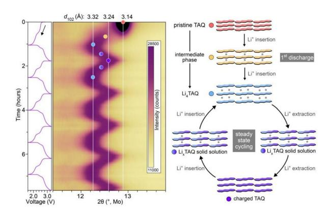
Structural evolution of TAQ during charge/discharge. In-operando PXRD patterns in the region of the (102) reflection and the corresponding voltage profile of a TAQ cell in LiTFSI/DOL/DME cycled five times at 200 mA g<sup>-1</sup>. A diagram representing the phase transformation mechanism of TAQ during cycling at 1C is shown to the right. Credit: *ACS Central Science* (2024). DOI: 10.1021/acscentsci.3c01478
