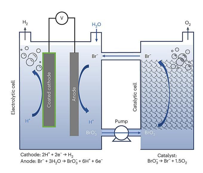
Proposed DWE process. Schematic illustration of the proposed DWE process with continuous generation of  $H_2$  and  $O_2$  in separate electrolytic and catalytic
