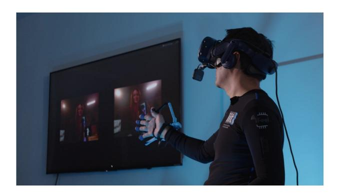
The iCub3 robot avatar system has been designed to facilitate the embodiment of humanoid robots by human operators encompassing aspects such as locomotion, manipulation, voice, and facial expressions with comprehensive sensory feedback including visual, auditory, haptic, weight, and touch modalities. Credit: IIT-Istituto Italiano di Tecnologia
