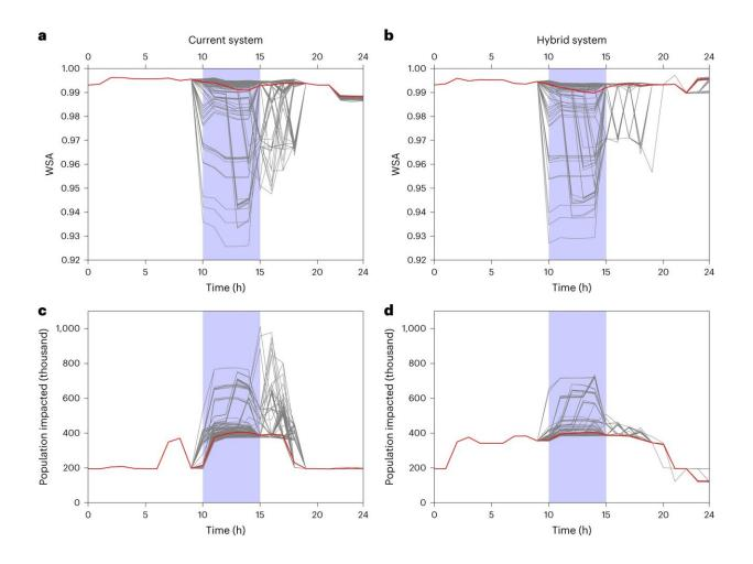
a,b: WSA index for all Pipe leak scenarios over the simulation period for current system (a) and hybrid system (b). c,d: Total population impacted (population with WSA
