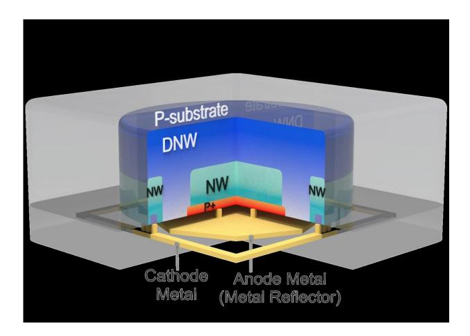
KIST single-photon avalanche diode developed in SK hynix's 40 nm backilluminated CMOS image sensor technology. Credit: Korea Institute of Science and Technology (KIST)
