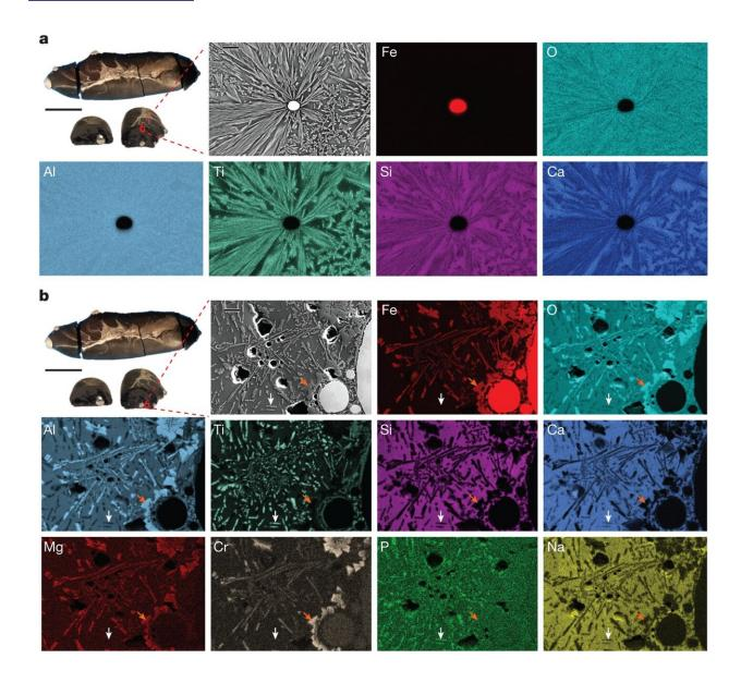
Microstructure of red mud after 10 min of processing with hydrogen plasma. Credit: *Nature* (2024). DOI: 10.1038/s41586-023-06901-z
