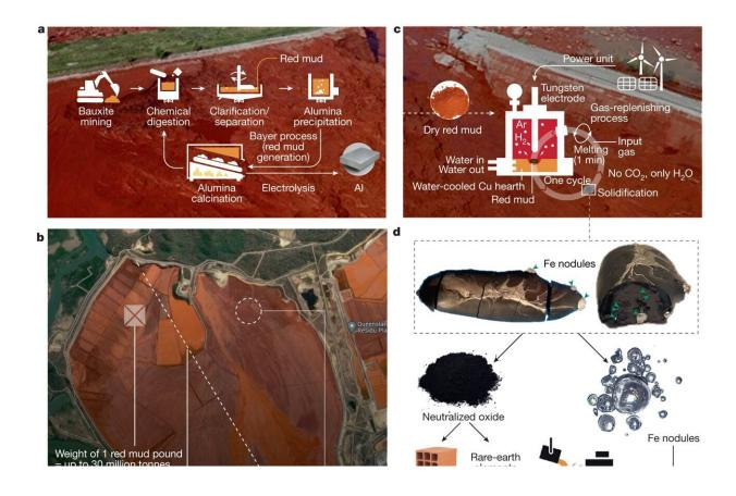
The generation, storage and hazards of red muds and solution with hydrogen plasma treatment. Credit: *Nature* (2024). DOI: 10.1038/s41586-023-06901-z
