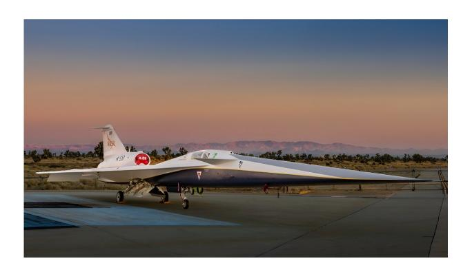
NASA's X-59 quiet supersonic research aircraft sits on the apron outside Lockheed Martin's Skunk Works facility at dawn in Palmdale, California. The X-59 is the centerpiece of NASA's Quesst mission, which seeks to address one of the primary challenges to supersonic flight over land by making sonic booms quieter. Credit: Lockheed Martin Skunk Works
