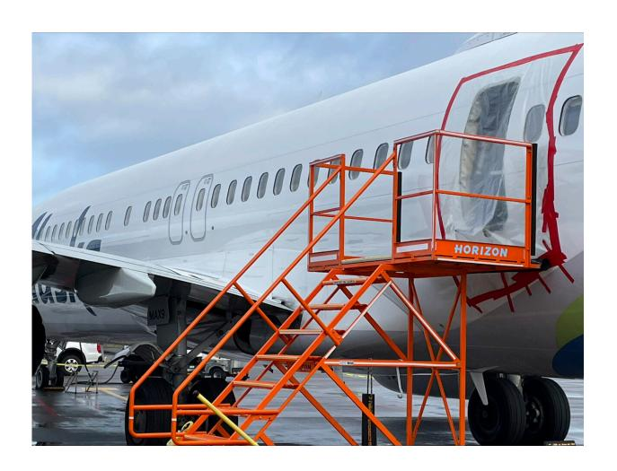
This image taken Sunday, Jan. 7, 2024, and released by the National Transportation Safety Board, shows a section of Alaska Airlines Flight 1282 that is missing panel on a Boeing 737-9 MAX in Portland, Ore. Federal officials are investigating Boeing's oversight of production of a panel that blew off a jetliner
