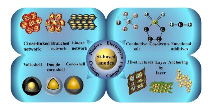
The importance of silicon-based anodes in lithium-ion batteries, emphasizing their improved performance through modifications involving binders, coatings, composites, and electrolytes. Credit: Li Wang, Jianping Yang, Donghua University, Shanghai, China
