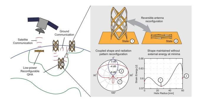
Operational concept of the multi-stable deployable and reconfigurable quadrifilar helix antenna for Disaster-Prone Areas. Overview of the coupled structural and electromagnetic reconfiguration used by the proposed low-power quadrifilar helix antenna for low-infrastructure areas. Credit: *Nature Communications* (2023). DOI: 10.1038/s41467-023-44189-9
