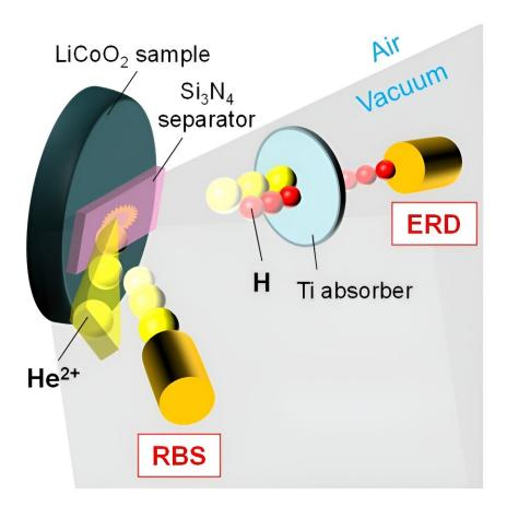
An oblique-view schematic image of simultaneous RBS and ERD analyses for a  $H_2O$ -uptake LiCoO<sub>2</sub> sample mounted on a sample holder in ambient air. Credit: Bun Tsuchiya
