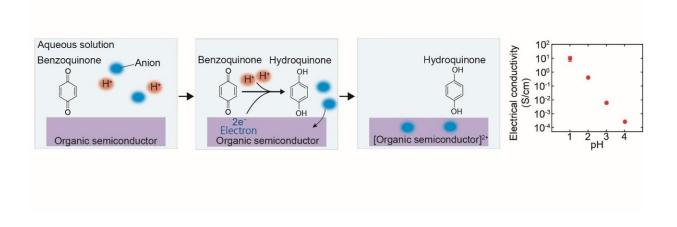
Schematics illustrating the mechanism of the newly developed chemical doping technique and a graph showing how changes in the pH of a solution can be used to control the doping levels of organic semiconductor thin films. Credit: Yu Yamashita National Institute for Materials Science
