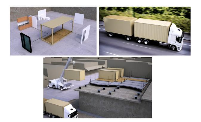
The components of modular housing are made in a factory and transported to the building site for assembly. Graphic illustration of modular construction methodology provided by UBC Smart Structures Lab, BC, Canada. Credit: Western Sydney University
