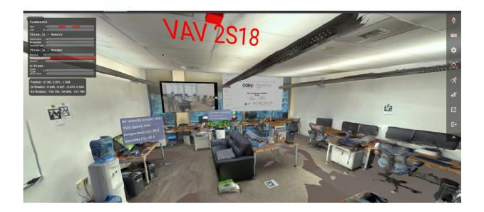
An example VR scene for an office with building hardware mapped as mixed reality objects that can be interacted with. Credit: University of California San Diego
