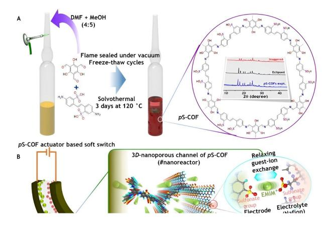
The synthesis and use of pS-COF as a common electrode-electrolyte host for electroactive soft fluid switches. A) The synthesis schematic of pS-COF. B) The schematic diagram of the operating principle of the electrochemical soft switch. C) The schematic diagram of using a pS-COF-based electrochemical soft switch to control fluid flow in dynamic operation. Credit: *Science Advances* (2023). DOI: 10.1126/sciadv.adk9752
