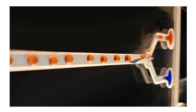
The separation of fluid droplets using a soft fluid switch at ultra-low voltage. Credit: *Science Advances* (2023). DOI: 10.1126/sciadv.adk9752
