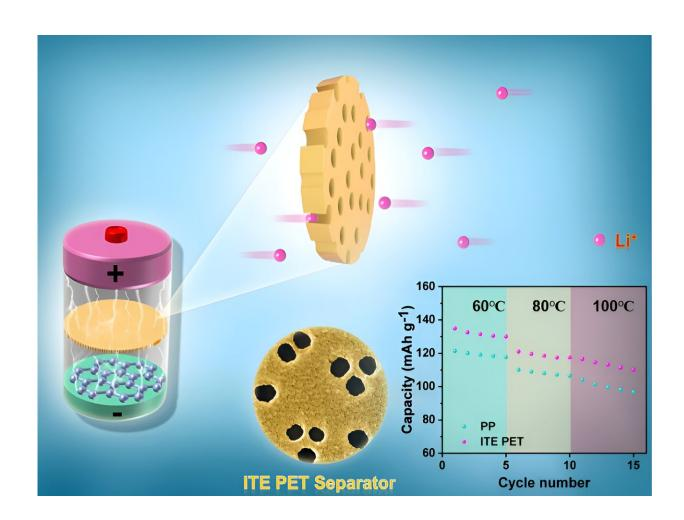
The SEM image and high-temperature cycle performance of the PET-based separator. Credit: IMP
