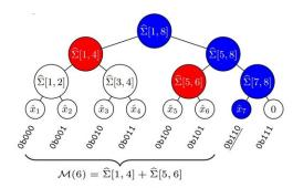
(b) Computation of  $\mathcal{M}(6)$  using Algorithm 1.
