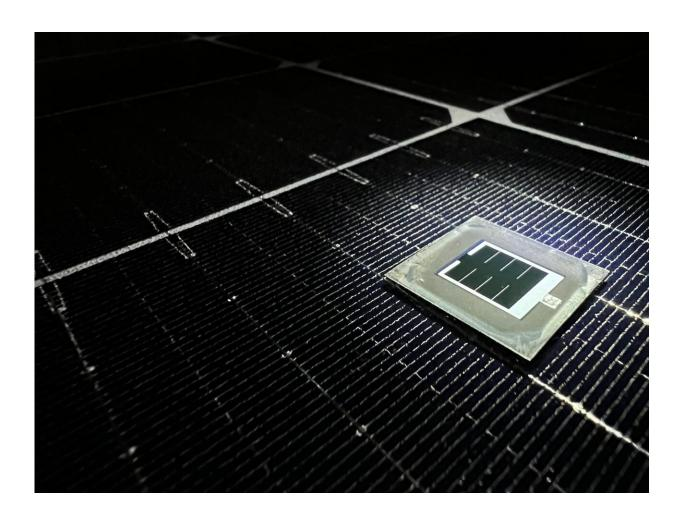
A perovskite/silicon tandem solar cell. Credit: 2024 KAUST
