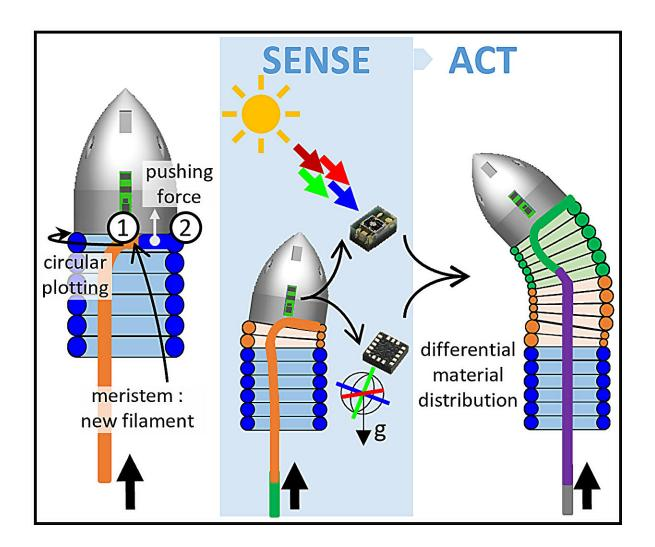
Schematic representation of the growing robot regions, their functionalities, and growth responses. Analogous to the shoot apex, the robot comprises sensing elements and a material deposition region localized at its head (points 1 and 2). In the meristem- like region, there is the addition of material and the generation
